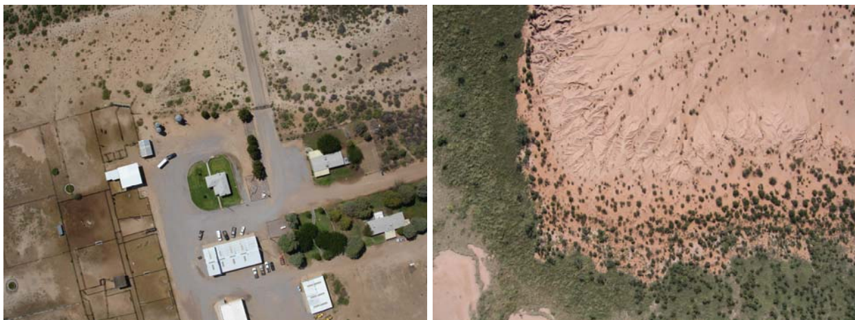
Figure 7. Images acquired from the modified model airplane (left) and from the BAT UAV (right) from 150 m above ground. Image extent is approximately 152 m x 114 m.
