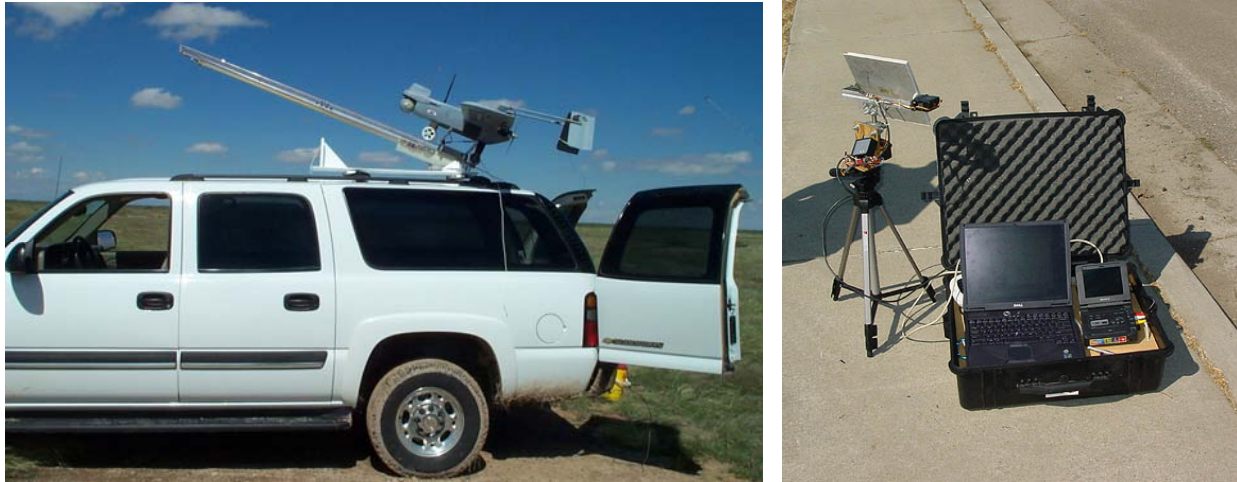
Figure 3. BAT 3 UAV on catapult launcher ready for takeoff (left). Ground station with laptop and video deck used for live video downlink, and telemetry antenna (right).
