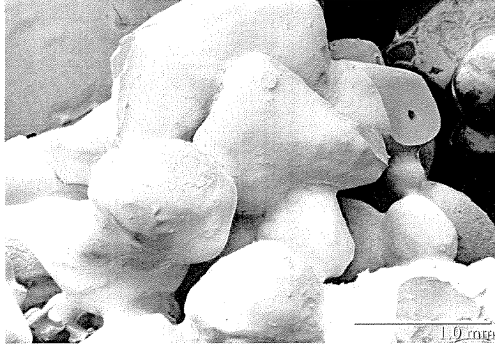
Fig. 4 Rounded snow grains from 2.5 m below the snow surface at site SP-1917.
