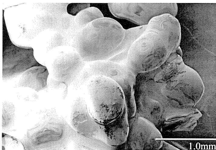
Fig. 3 Rounded snow grains from 10 cm below the snow surface at site SP-1841.
