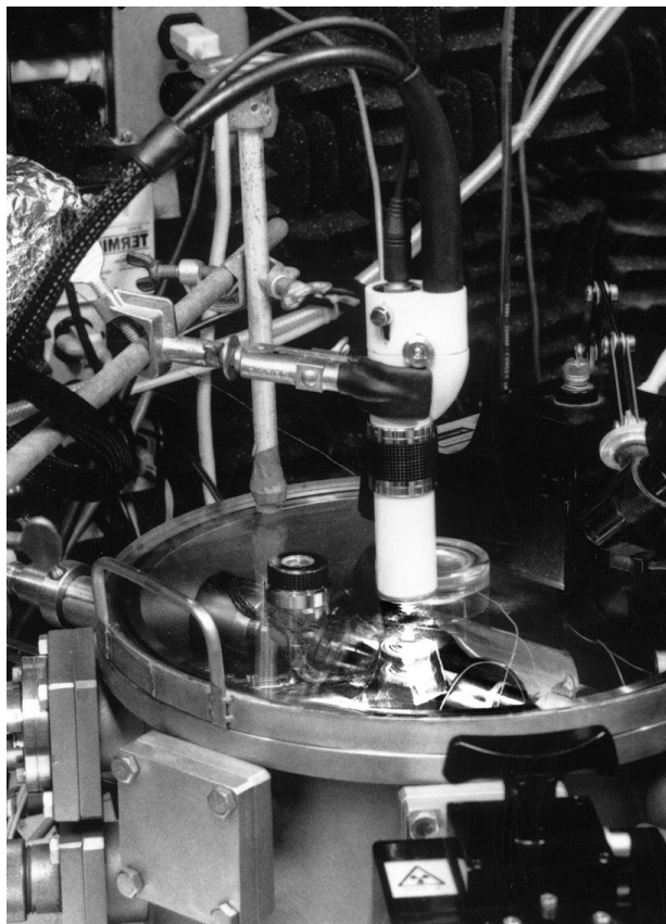
FIG. 2 Video microscope system that is interfaced to a monitor and computer as described above. The microscope is mounted above the clear glass cover on a modified Denton DFE-3 freeze-etch module. With this system, the sample is maintained under vacuum at -196^{\circ}\text{C} . The stage in the freeze etch-module allows the sample to be tilted through 180^{\circ} so that multiple views, including stereo pairs, can be obtained at different angles.
