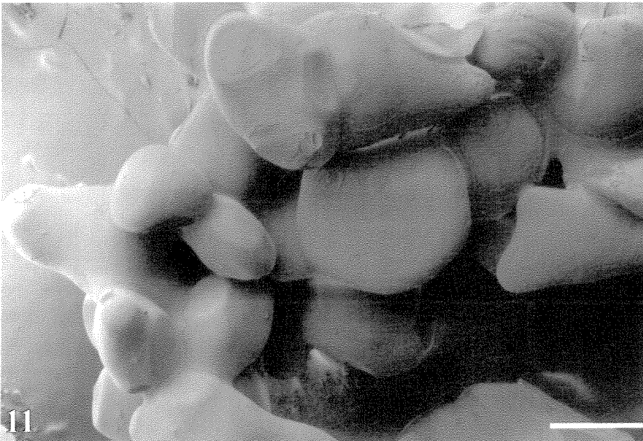
Fig. 11 Bonded and rounded snow grains from the middle layer of the melting snowpack at Loveland Pass, Colorado. This part of the snowpack had little visible liquid water and snow grains are not spherical. (Collected at a snowpack temperature of 0^{\circ}\text{C} ; stored for 7 days in a Dewar flask; magnification 30\times ; bar = 0.5 mm).
