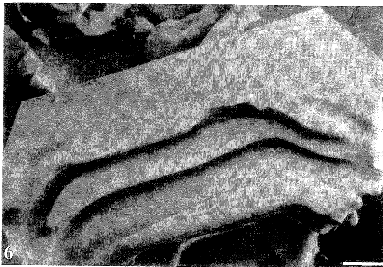
Fig. 6 Layered crystal indicative of depth hoar from the bottom layer of the Berthoud Pass, Colorado snowpack. (Collected at a snowpack temperature of -3^{\circ}\text{C} ; stored for 5 days in a Dewar flask; magnification 30\times ; bar = 0.4 mm).
