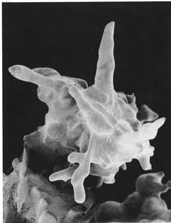
FIG. 19 At more advanced stages of melting, the individual snow crystals are no longer distinguished. The particle consists of a highly amorphous mass without any crystalline faces. (Collected at 0°C, imaged at 5 kV.) Horizontal field width = 1.6 mm.
