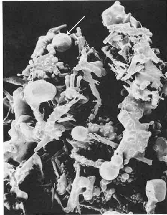
FIG. 18 Snowflakes consisting of aggregations of partly melted snow crystals held together in an amorphous matrix. Several microspheres (arrows) are associated with the surface of the melting snowflake. (Collected at 0°C, imaged at 5 kV.) Horizontal field width = 4.0 mm.
