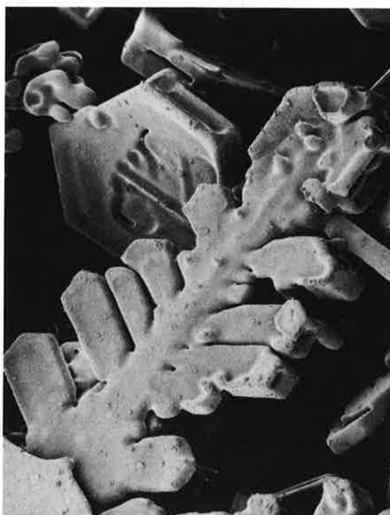
FIG. 15 Branched end of metamorphosed dendritic crystal shown in Figure 14. The surface of the "crystal" appears to flow from one face to the next rather than forming sharp angular intersections. (Collected at 0°C, stored for 1 month in LN 2 , imaged at 5 kV). Horizontal field width = 1.0 mm.
