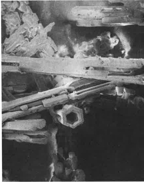
FIG. 11 Needles consist of long slender columns that frequently have a hollow core. The needles generally are associated in irregular bundles. (Collected at -6^{\circ}\text{C} , imaged at 5 kV.) Horizontal field width = 1.1 mm.
