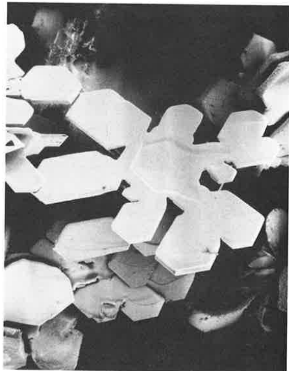
FIG. 4 Irregularly shaped snow crystals are far more common than the symmetrical forms. However, even though the branches are nonsymmetrical, they do exhibit variations of the hexagonal plates. (Collected at -5^\circ\text{C} , imaged at 5 kV.) Horizontal field width = 1.8 mm.
