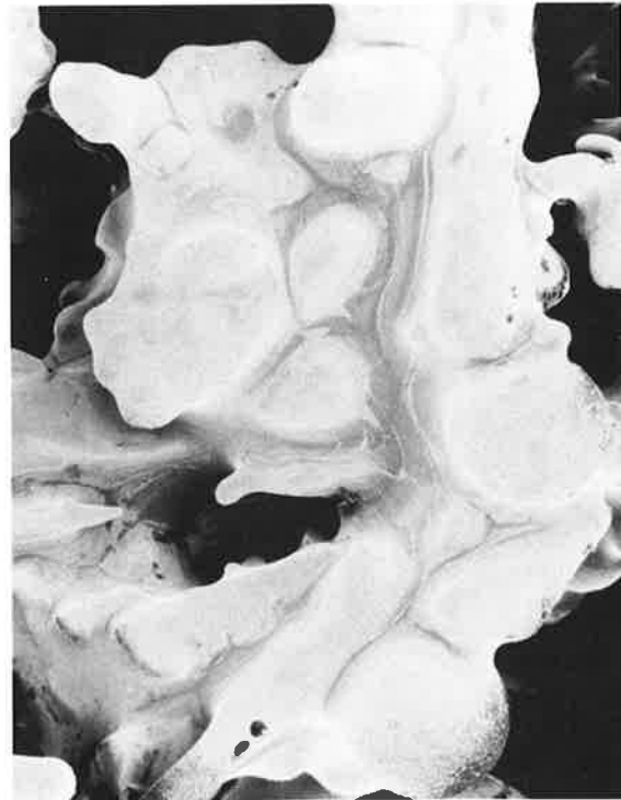
FIG. 20 At the most advanced stage of melt-freeze, the wet snow consists of an aggregation of spherical masses that have no crystalline characteristics. (Collected at 1°C, imaged at 5 kV.) Horizontal field width = 1.4 mm.
