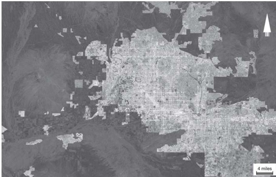
Fig. 3. Impervious fraction layer of the Phoenix metropolitan area. White = 100%; black = 0%.
