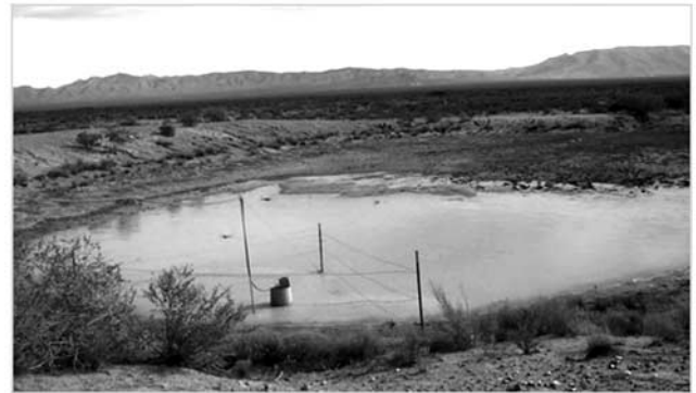
Figure 2. Typical stock tank with water discharge measurement equipment after an overland flow event in the Jornada Basin.
