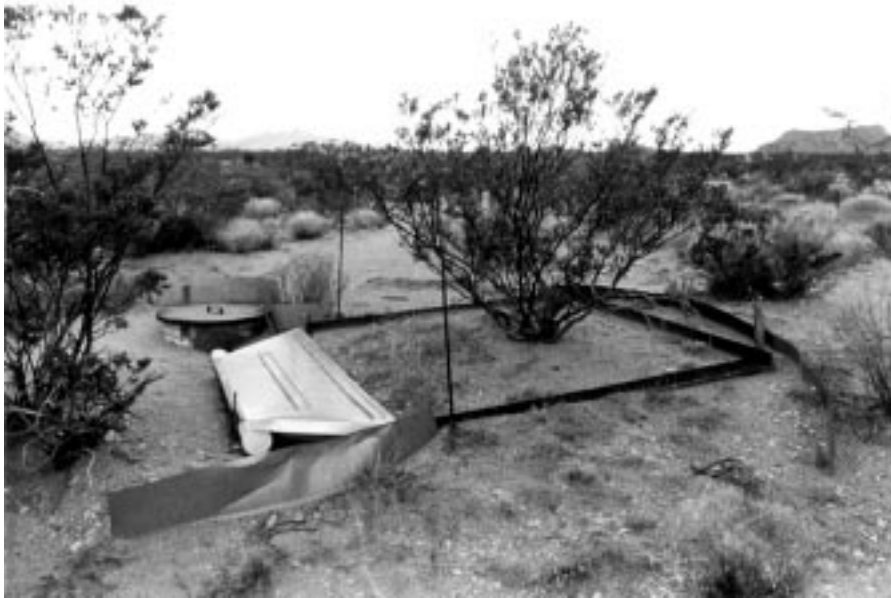
Figure 1. Runoff plot located in creosotebush shrubland of the Jornada Basin, New Mexico. The edges of the plot are 2 meters in length. Photograph by David Hamilton.
