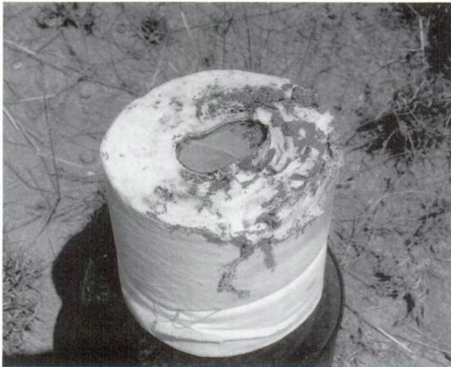
Figure 6.10. Bait roll showing surface galleries and paper eaten by subterranean termites.
