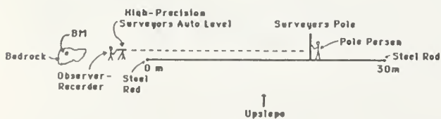
Figure 4. Diagram of the setup for surveying soil-surface levels along a permanent line transect relative to a benchmark (BM).
