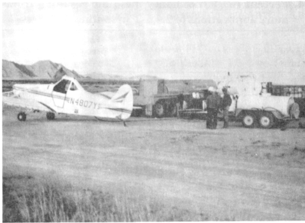
Fig. 4. Equipment for mixing the spray solution and loading the aircraft to minimize time on the ground for the aircraft. The equipment includes water tanks with a pump, diesel and herbicide with barrel pumps that accurately measure liquids, and a mixing-loading tank equipped with a pump. The mixing-loading tank has both paddle and by-pass agitation to keep the oil and water phases of the spray solution properly mixed.
