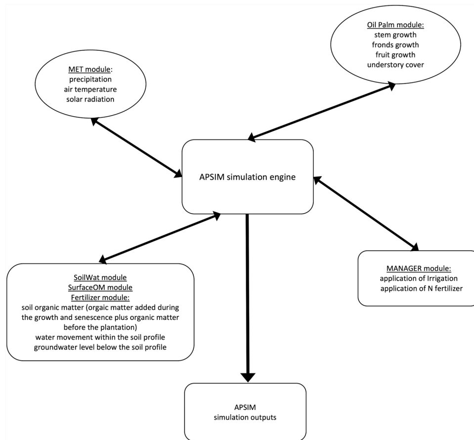
Fig. 2. Flow diagram showing the different modules of the APSIM model interacting through a central simulation engine as applied to an oil palm plantation growing on marginal lands.
