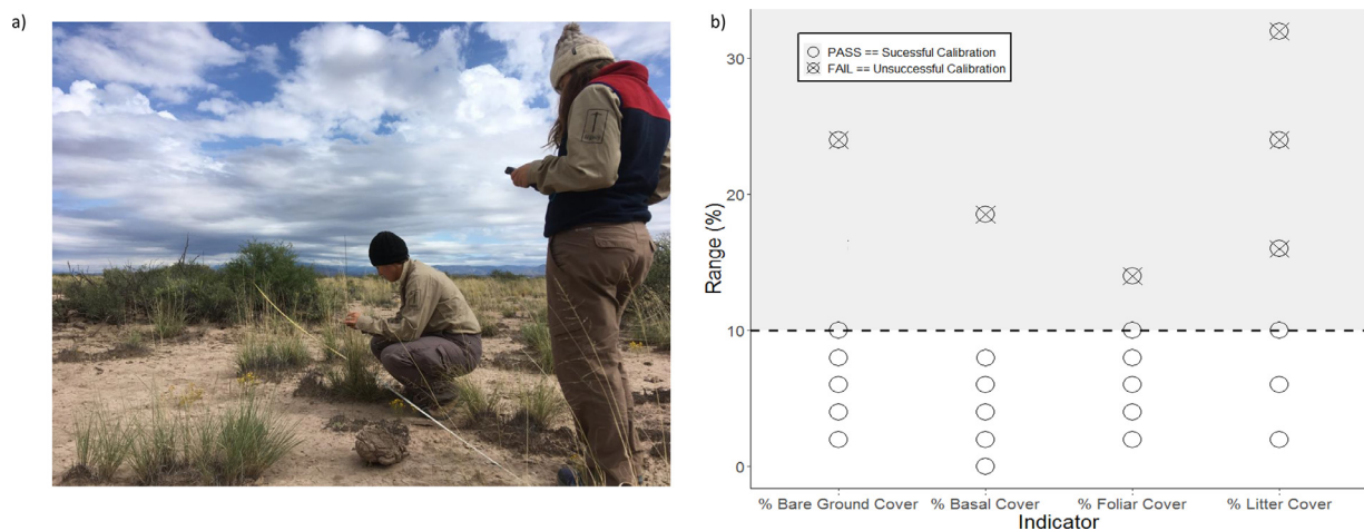
Figure 3. Calibration (Question 7) is an important process to minimize observer variability in the line-point intercept method (A), especially when the true value is not known or is difficult to measure. 12 For successful calibration in the BLM AIM and the NRCS NRI programs, the line-point intercept absolute range of variability among observers should be less than or equal to 10% (B). 12,50 Photo courtesy of Rachel Burke
