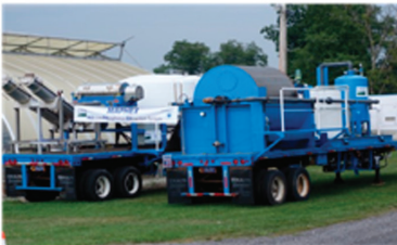
Fig. 5. Examples of on-farm and mobile treatment systems developed in the United States to recover phosphorus from liquid dairy and swine manures.
