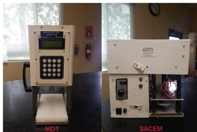
Fig. 3. Photograph of Mohr Digi-Test (MDT) and soil-aggregate crushing-energy meter (SACEM).
