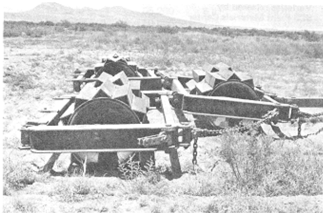
Converted rolling chopper imprints a 21-foot width.
