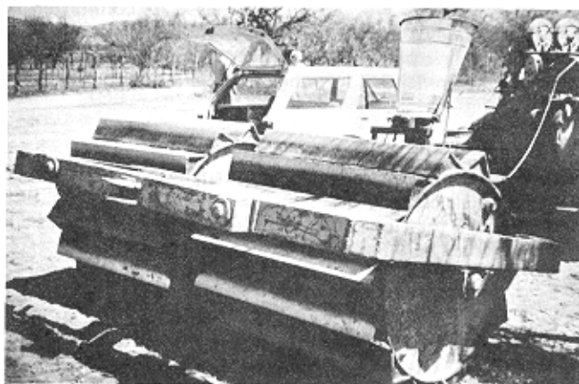
Converted sheepfoot roller imprints a 9-foot width.
