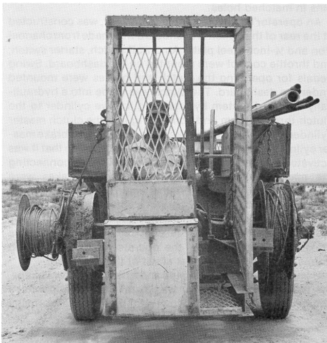
Protected by a steel cage, pulling rig operator has a clear view of well head. The 12-inch, heavy duty winch drum on left holds 150 ft of \frac{3}{8} -inch cable and the wheel to which it is attached holds 150 ft of reserve cable. The winch drum on the right holds 700 ft of \frac{3}{8} -inch cable and is used in baling and other light load operations.
