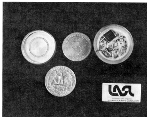
Fig. 5. The hybrid radio transmitter developed at LASL shown with battery and Kel-F case.
