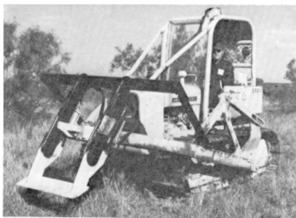
Low-energy grubber with hydraulic attachment to adjust cutting blade angle for improved soil penetration and stump splitting.
