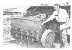
This equipment converts the cover on sites dominated by worthless brush to useful plants, in a onceover pass. It grubs undesirable brush, forms basins to catch water, prepares the seedbed and seeds desirable species, and deposits shade on the seeded area. The seeder (right) places seed in a firmed seedbed, and drag chains cover it lightly.
