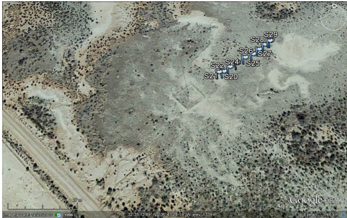
Fig. 2. Configuration of the array, image courtesy of Google Earth. The GPS location of S29 appears slightly inaccurate – its separation from S28 was similar to the other spacings (see Fig. 3). The dirt road providing access is visible at lower left; an instrumentation tower and square fence is visible in the center.
