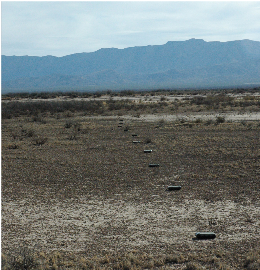
Fig. 3. Field photograph of the array configuration. The logger boxes are approximately 20 cm long, spaced by about 4 m. Note that the surface is partly grass-covered.
