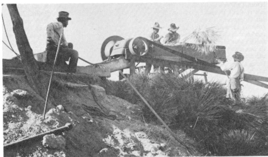
Ensilage machine in operation, chopping and shredding soapweed stems and leaves. (U.S. Forest Service photo, 1916.)
