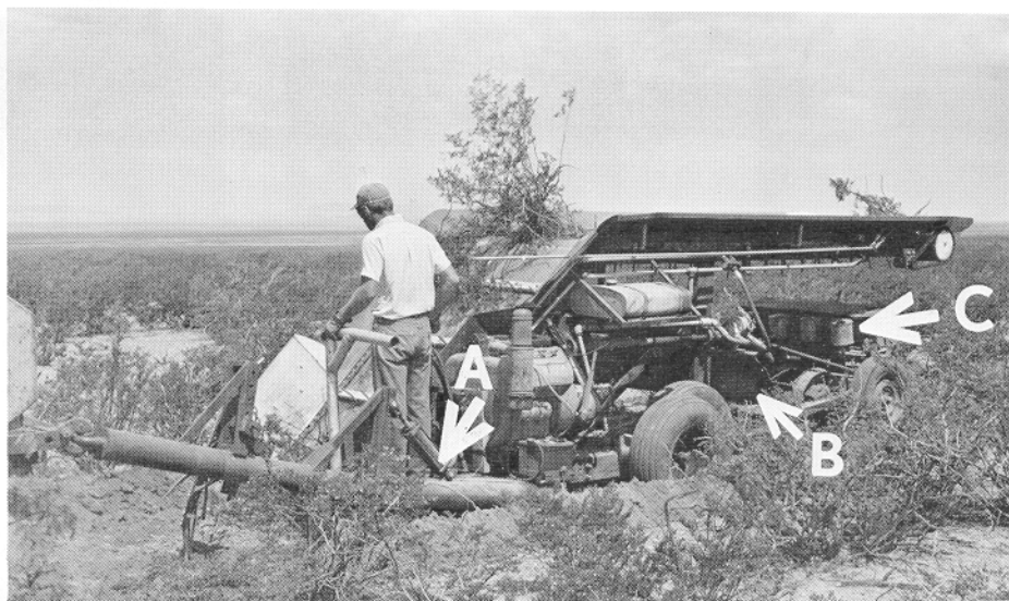
Fig. 5. Final version of conveyor having pickup height adjustment (A), basin-forming blade (B), and low profile planter (C).
