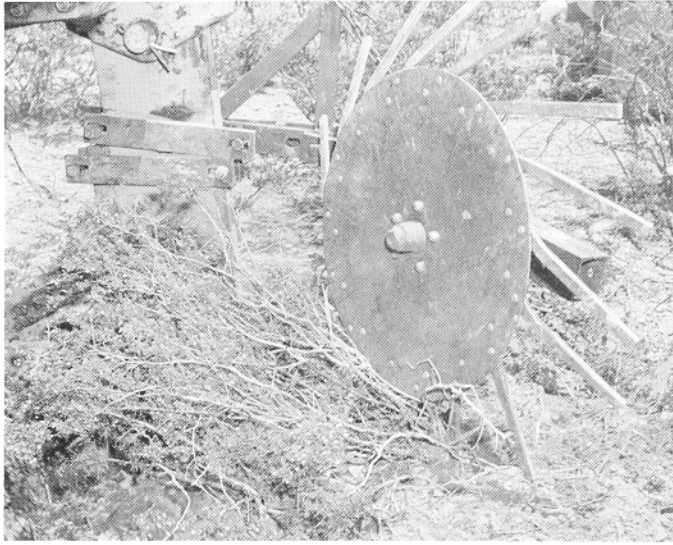
Fig. 2. One of two side delivery rake wheels used to windrow the brush for conveyor pickup.
