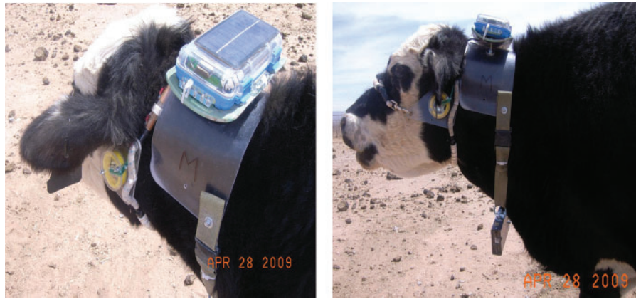
Fig. 1. Cow wearing a stretch-halter/neck saddle electronics package. GPS hardware is housed inside the rectangular box equipped with solar panels. Continuous power is supplied from a battery located inside a box hanging below the cow's neck. A plastic ring below the left ear and two metal cylinders behind it, separated by a white insulator, can provide sound and electrical simulation cues, respectively, when activated (Directional Virtual Fencing; DVF™; Anderson 2007). No cues were activated in this study.
