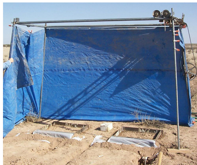
Fig. 1. Rainfall simulator used for all treatments. Nozzle is moved across plots using a metronome-timed hand-operated pulley system.
