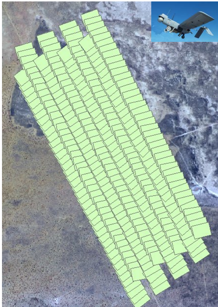
Figure 6. Footprints of BAT UAV imagery overlaid on Quick Bird image.
