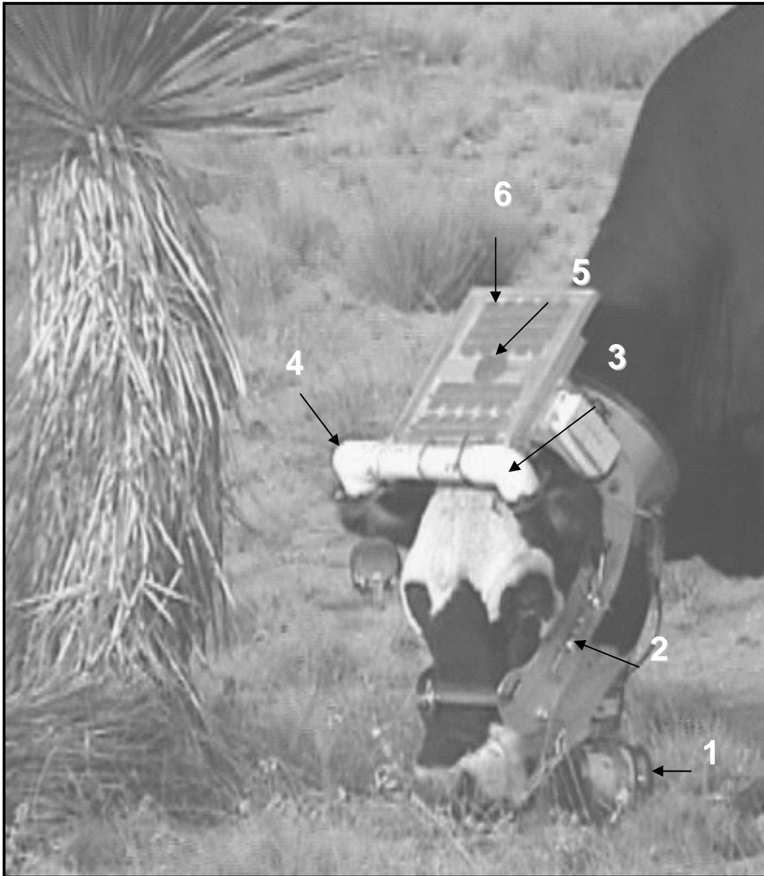
Figure 8. A grazing cross-bred beef cow wearing a battery (1) powered Directional Virtual Fencing (DVF™) device equipped with spring loaded electrodes (only left side pair shown 2) for providing electrical stimulation and left (3) and right (4) piezo speakers housed inside Poly Vinyl Chloride (PVC) pipe for audio stimulation. A Global Positioning System (GPS) antenna (5) is located in the centre of a panel of solar cells (6). This prototype platform may appear clumsy but was remarkably robust during numerous field trials conducted between 2001 and 2005.
