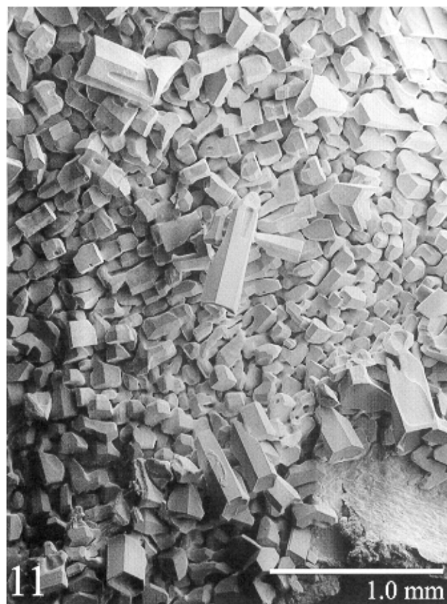
Fig. 11. Surface hoar or frost, consisting of a dense aggregation of irregular crystals and a few short columns that formed by vapor deposition on the surface of a blade of grass. Frost samples forming on biological or non-biological substrates can be mounted on specimen plates and frozen in \text{LN}_2 to preserve their structural integrity. Sample collected in West Virginia.
