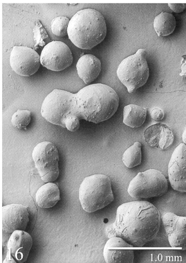
Fig. 16. Newly formed artificial snow collected from a plume generated by a snow gun in Vermont. Artificial snow forms when water, generally at temperatures less than -3^\circ\text{C} , is atomized under pressure. The minute droplets, which quickly freeze before reaching the ground, can vary in size from 0.1 to 1.0 mm as a function of the pressure and type of gun that was used to atomize the water.
