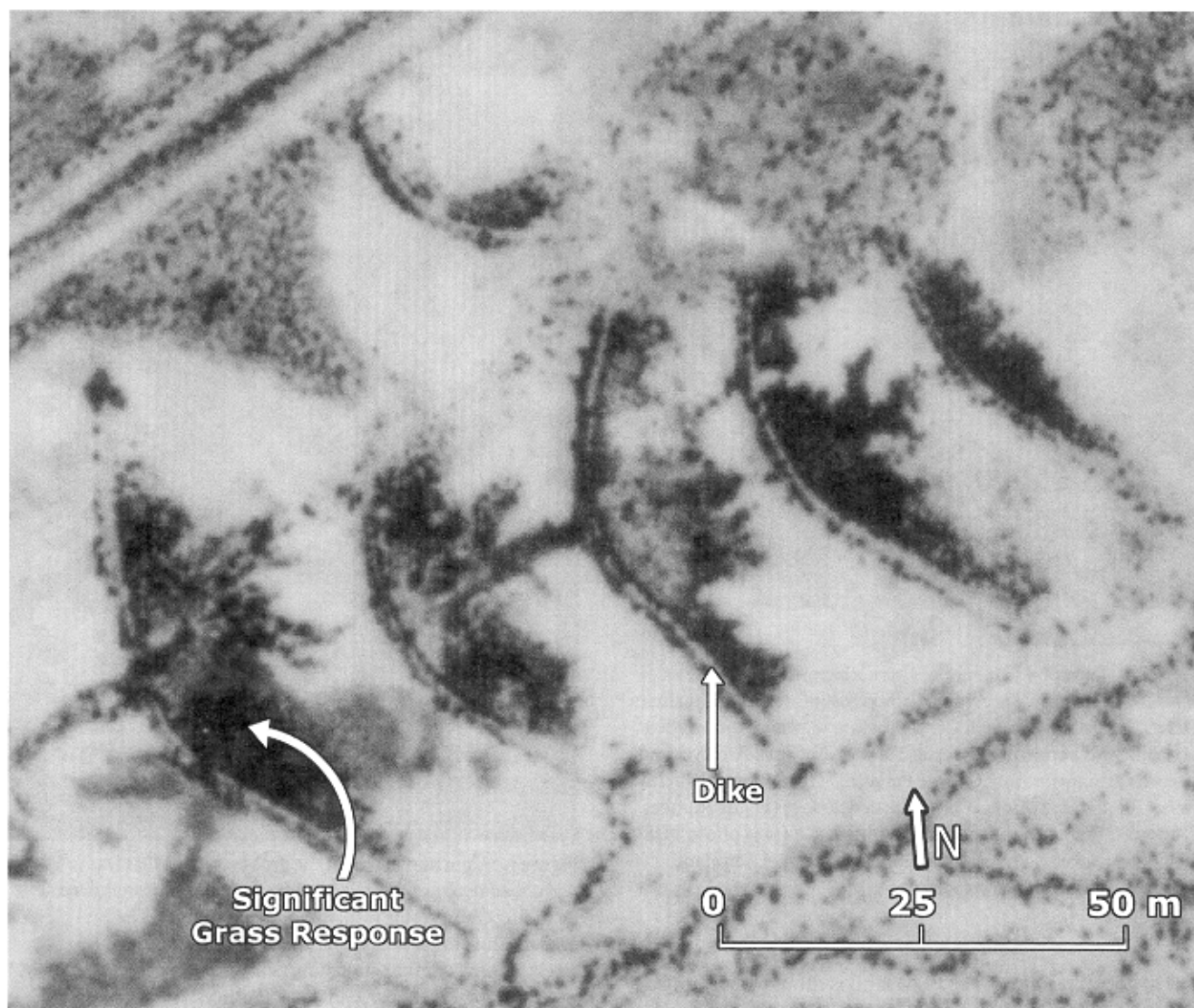
Figure 5. 1994 aerial photograph of water ponding dikes on the Jornada Experimental Range near Ace Tank; these were established in 1975. The photo indicates a positive vegetation response to treatment. (Source: US Environmental Protection Agency.)
