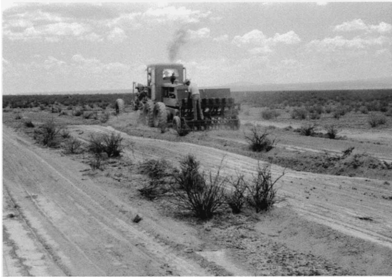
Figure 10. Road grader and grass seeding equipment operating in tarbush area of JER pasture 6 in 1964.
