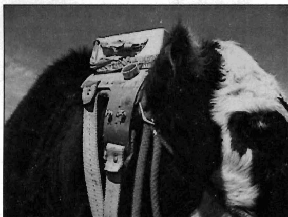
Figure 3 Virtual fence device housed in a neck-saddle worn by a haltered cow. Above the front strap securing the neck-saddle around the animal's neck are a pair of horizontally-spaced, spring-loaded electrodes for administering electric shock cues to the animal's right side and directly above them is the piezo transducer, housed in a protective cylinder, for producing audio sound cue(s). Electronic hardware and software, with batteries for power, are housed in the rectangular box sitting on the saddle.
