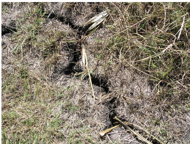
Figure A1-34. Shrink-swell behavior of Vertisols at the Grassland, Soil and Water Research Laboratory (GSW) results in formation of cracks in the soil, with consequences for ecosystem dynamics, agricultural management, and building and road foundations. (Photo by R. Daren Harmel.)
