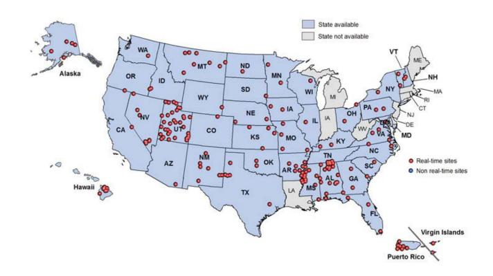
The Soil Climate Analysis Network consists of automated remote sites which collect soil moisture and soil temperature data along with precipitation, wind, and solar radiation data. These sites are located throughout the United States and other global locations. These data are used for the management and prediction of climatic issues affecting our natural resources.
