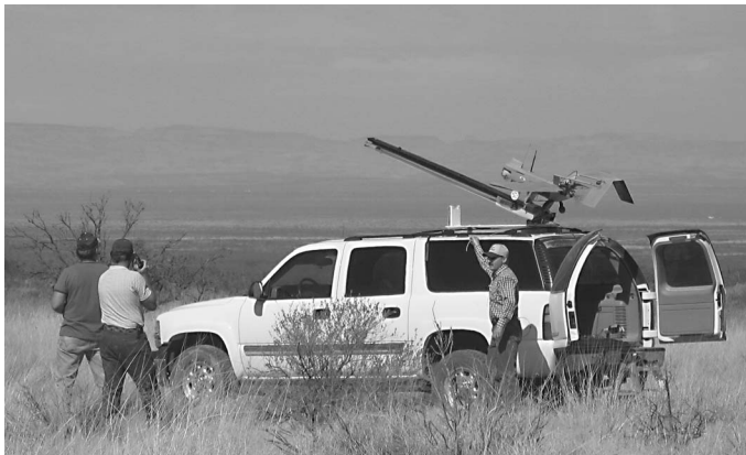
Figure 1. BAT 3 UAS ready to be launched from the catapult. One person holds the launch cord, the second person is on stand-by for manual control, the third person serves as visual observer and performs radio communications.
