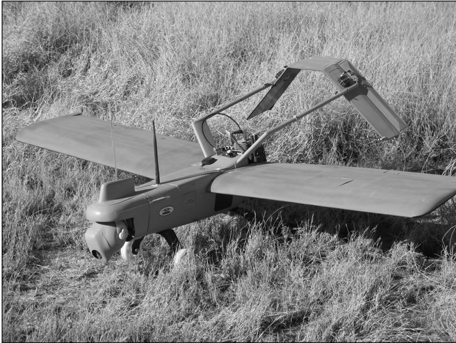
Fig. 3. BAT 3 UAS. The digital camera is mounted in the left wing, and the video camera is in the nose of the aircraft.
